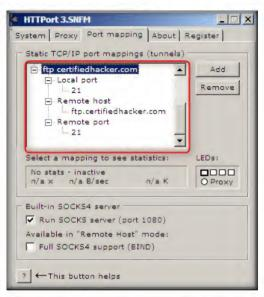
FIGURE 4.8: HTTPort Static TCP/IP port mapping
